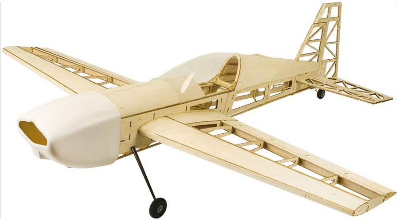
Image: The EXTRA330 airframe in a partially assembled state, showing the balsa and plywood structure before covering.
