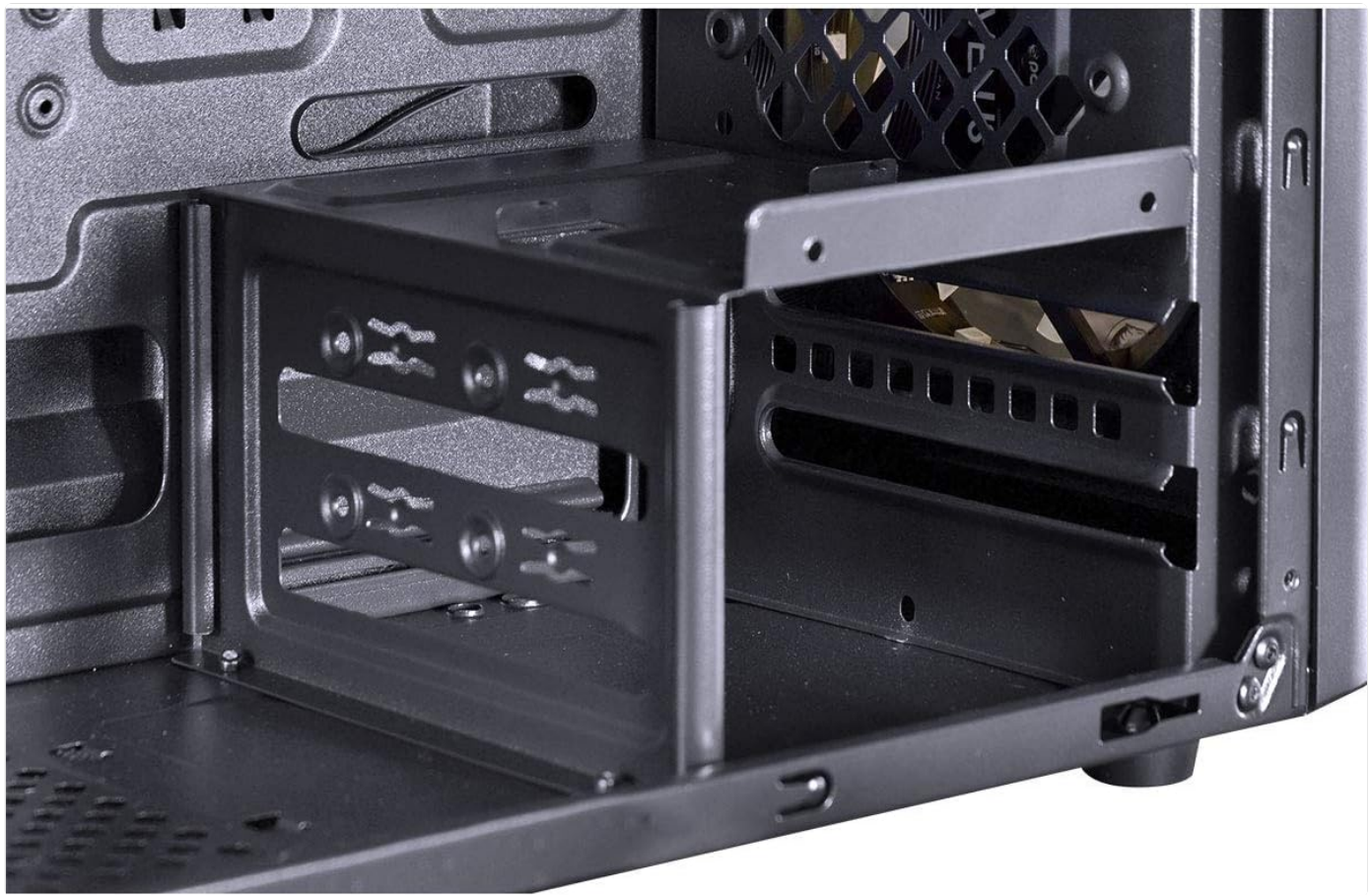
Image 6.2: Drive cage for 3.5-inch hard drives.
