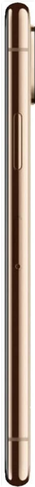
Figure 3: Side view of the iPhone XS Max, showing the stainless steel band and side button.
