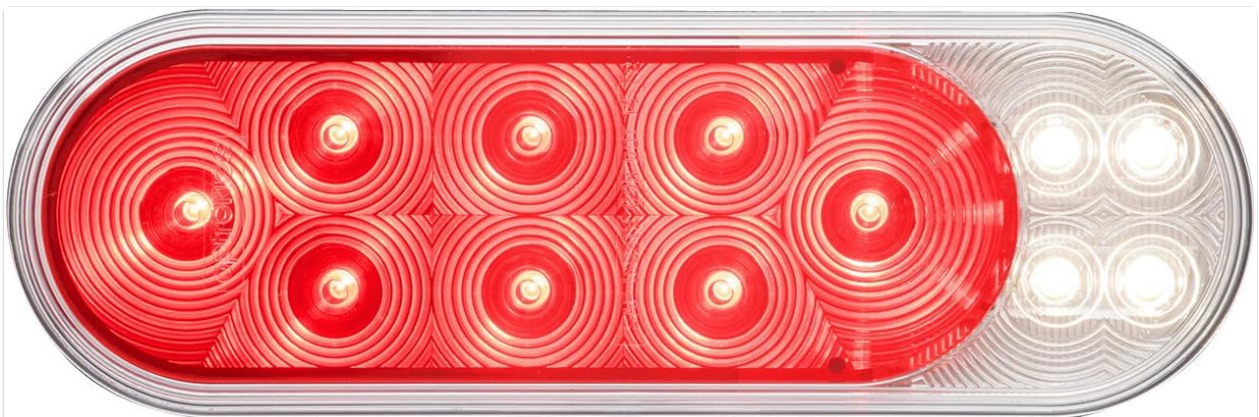
Figure 5.1: Optronics LED Fusion Tail Light illuminated. This image shows the red stop/tail/turn section brightly lit, along with the white back-up light section illuminated.
