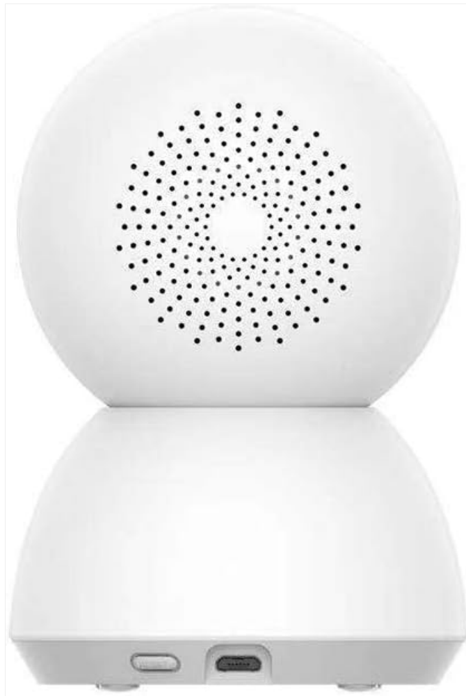
Figure 3: Rear view of the camera, showing the speaker grille and USB power port.
