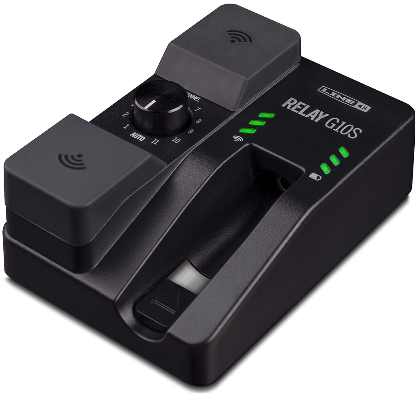
Figure 4.2: The G10T transmitter with its green status LED indicating active connection or charge status.
