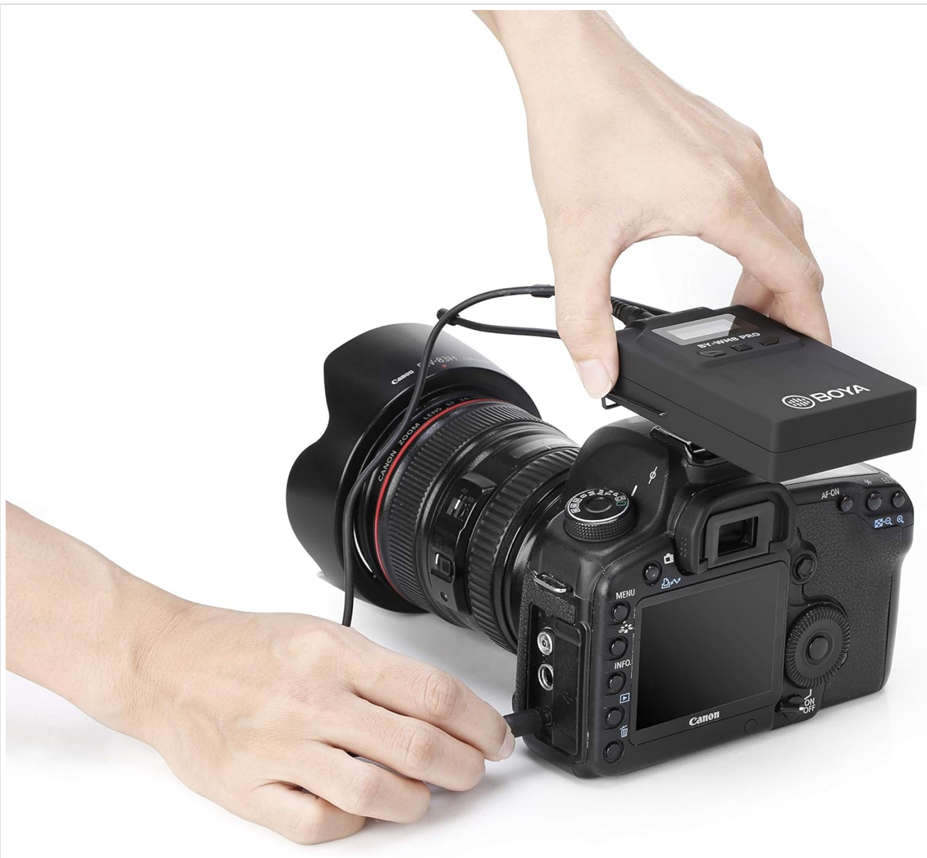
Figure 4.2: Connecting the receiver to a DSLR camera's audio input.
