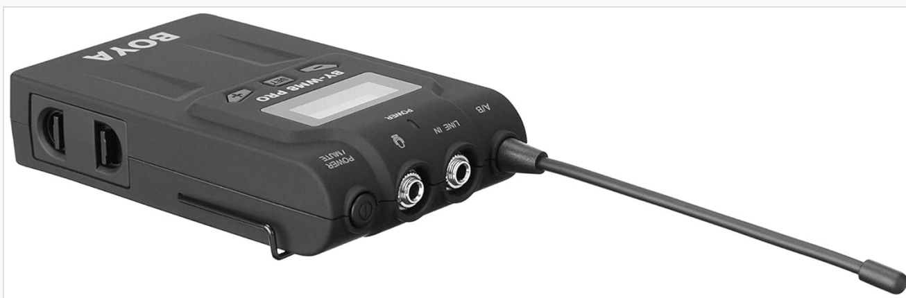
Figure 3.2: Top view of a BOYA BY-WM8Pro-K1 unit, illustrating the various ports and controls.
