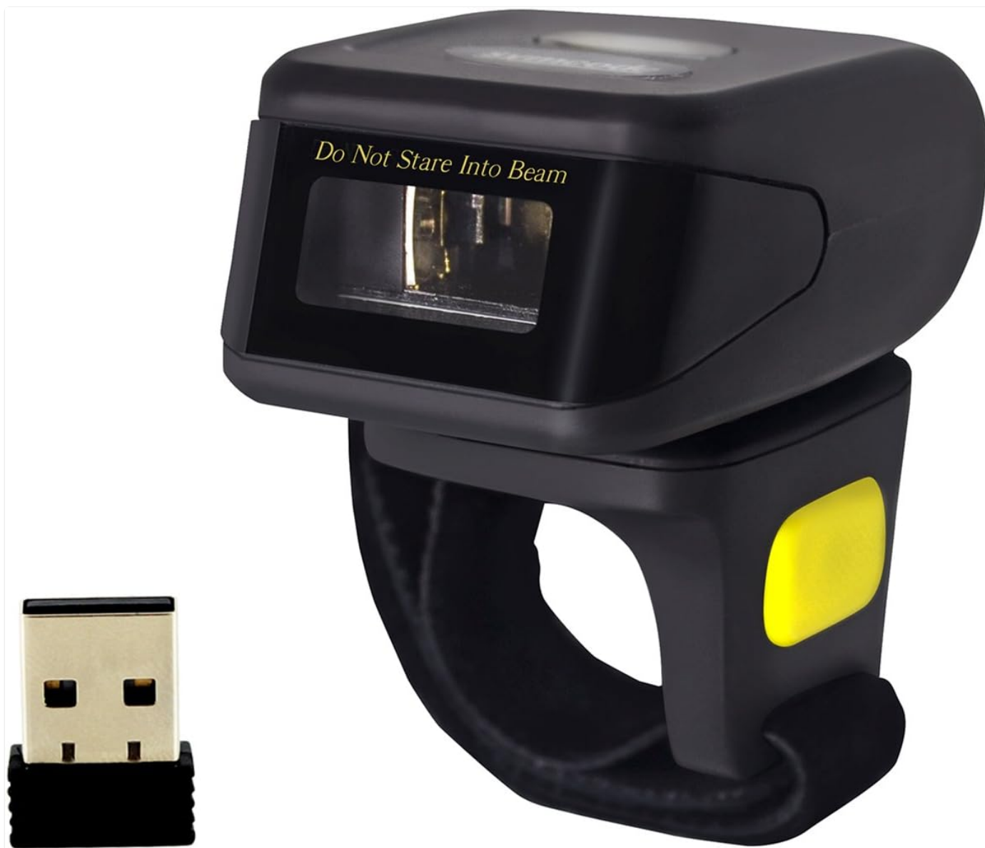
Image: The Symcode ring barcode scanner shown alongside its USB dongle, illustrating its compact form factor and connectivity option.
