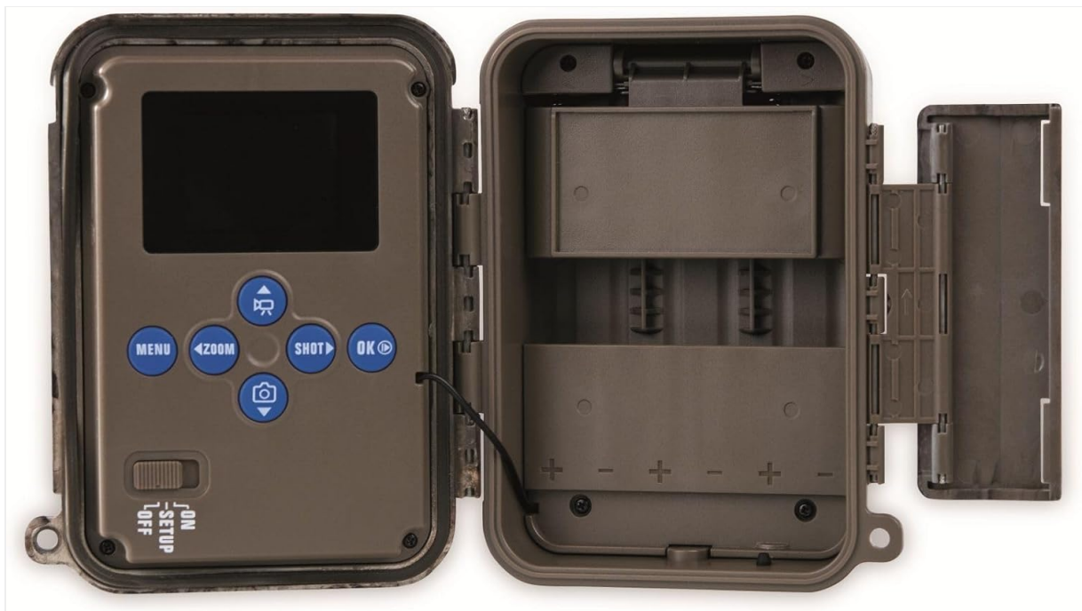
Image: Inside view of the camera, displaying the battery compartment on the right and the control panel with screen and buttons on the left.
