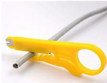
2. Put the wire into stripper tool and cut the skin.
