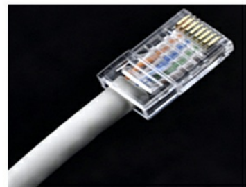
6. Ensure all pins are set, use tester tool to check .
