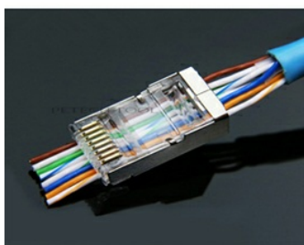
4. Insert wires into the connectors.
