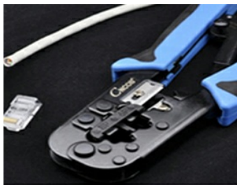
1. Prepare the connectors crimper, and the wires.
