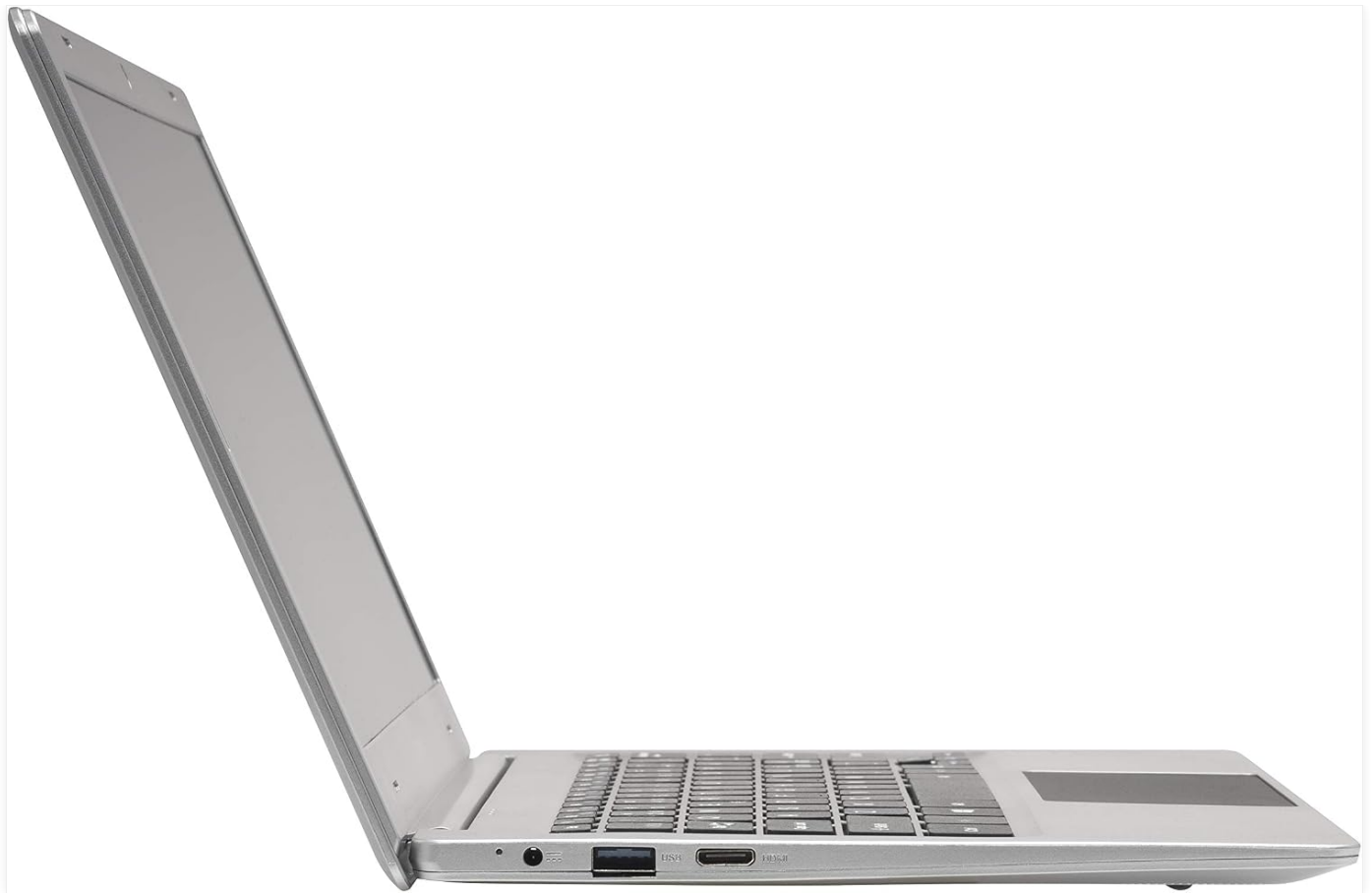
Figure 2: Left side of the laptop. This view highlights the various ports available on the left side, including the power input, USB ports, and possibly an HDMI port, crucial for connecting peripherals and charging.
