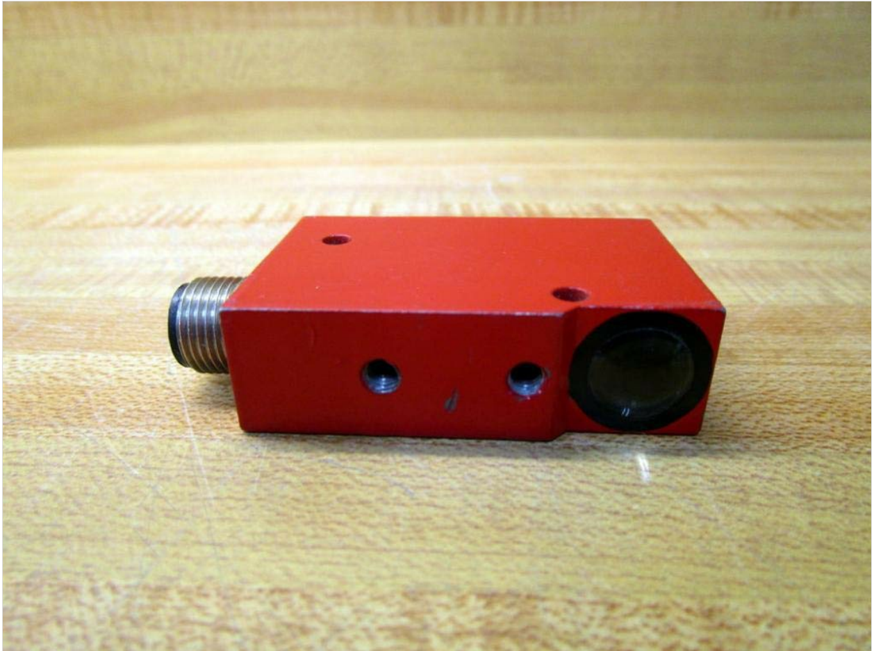
Figure 4.1: View of the sensor's front face, showing the optical lens for light emission and reception. Proper alignment with a reflector is crucial for operation.
