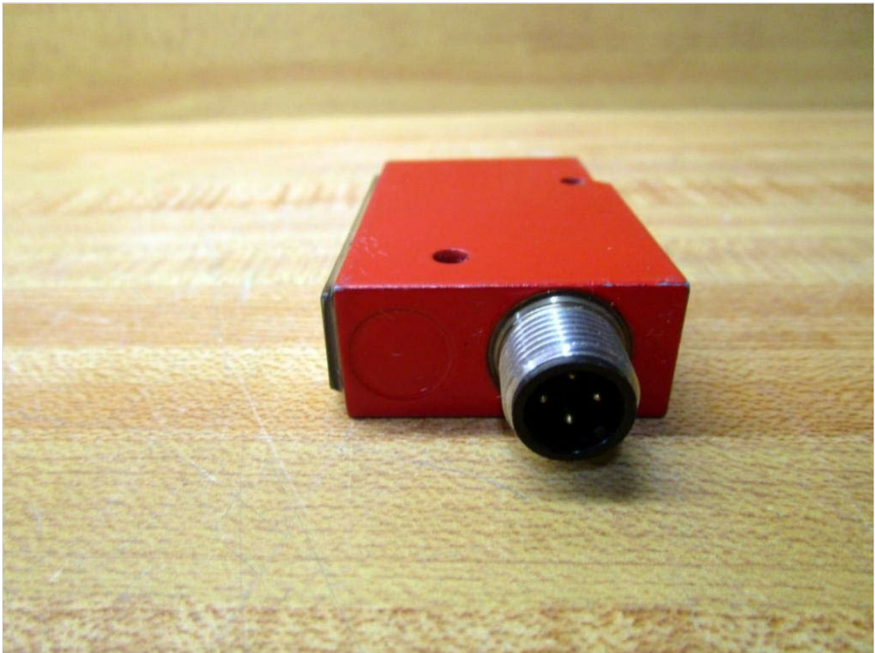
Figure 4.3: Close-up view of the M12 electrical connector on the sensor. This connector provides a robust and reliable
