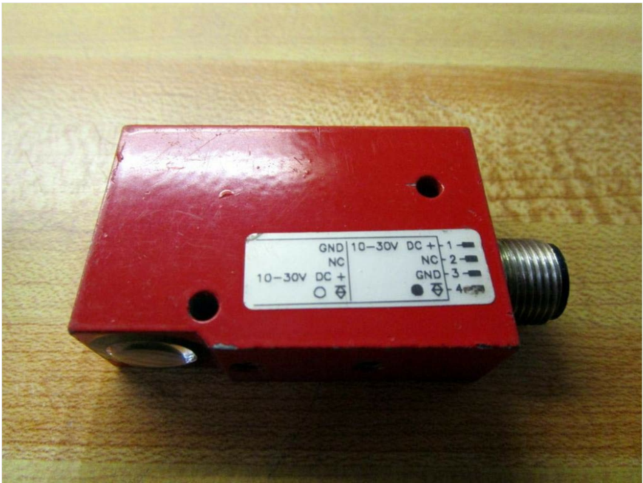
Figure 4.2: Wiring diagram for the LEUZE PRK-18/4-DL.4 sensor. It shows the M12 connector pinout: Pin 1 (Brown) for 10-30V DC+, Pin 3 (Blue) for GND, Pin 4 (Black) for PNP LO/DO output. Pin 2 (White) is NC (Not Connected).
