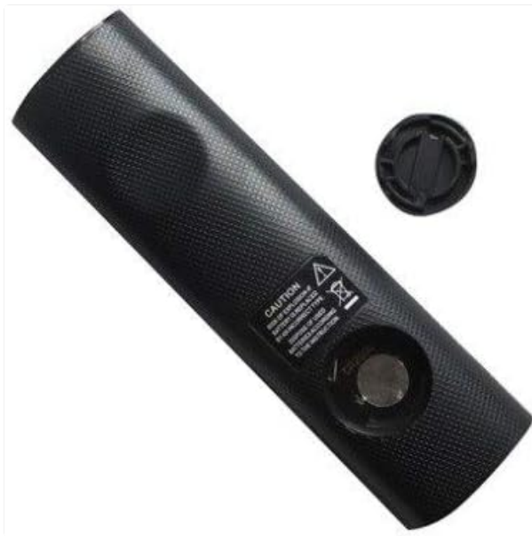
Figure 1: Back view of the remote control with the battery compartment. The circular cover indicates where the CR2032 battery is inserted.
