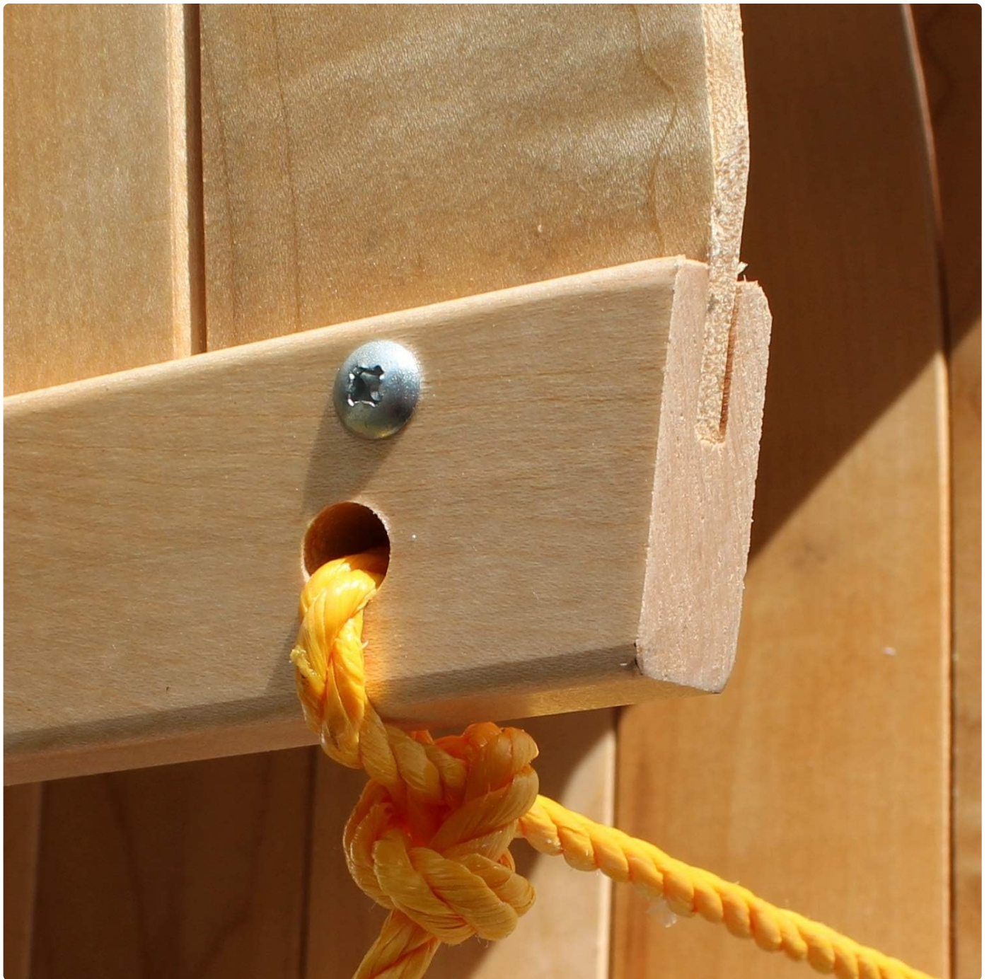
Image: A detailed view of the tow rope attachment point on the front of the toboggan, showing how the rope is secured through the wooden frame.
