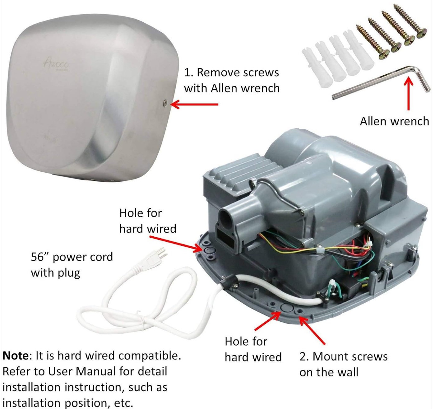
Figure 2: Installation steps for the Awoco Hand Dryer.
