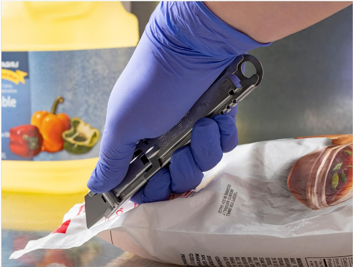
Figure 5.1: Proper technique for using the OLFA SK-14 to cut packaging.
