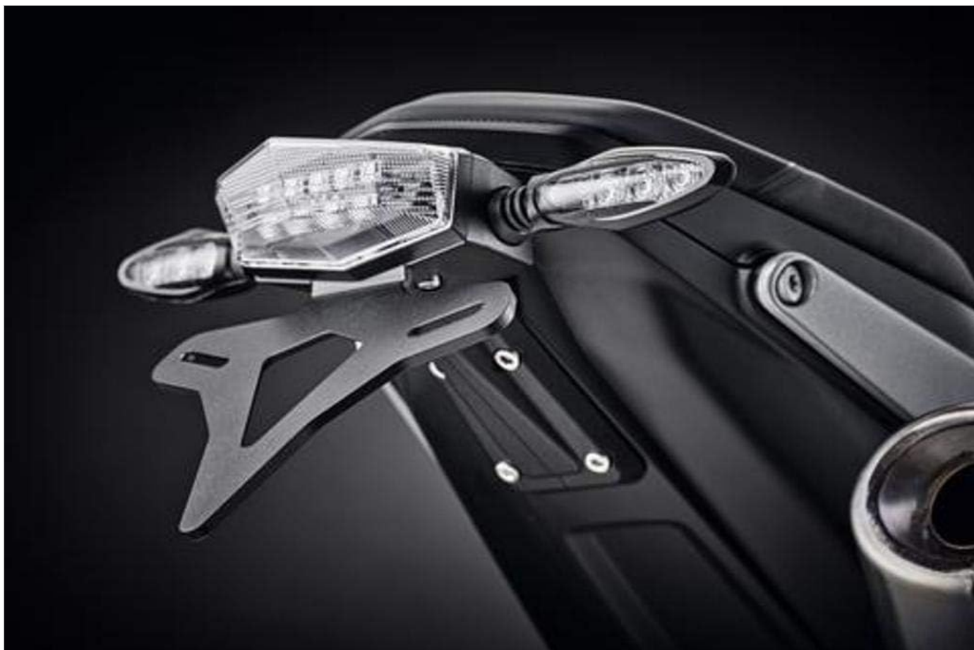
Figure 2: Rear view of the tail tidy installed on a KTM Duke motorcycle, showcasing its compact design.
