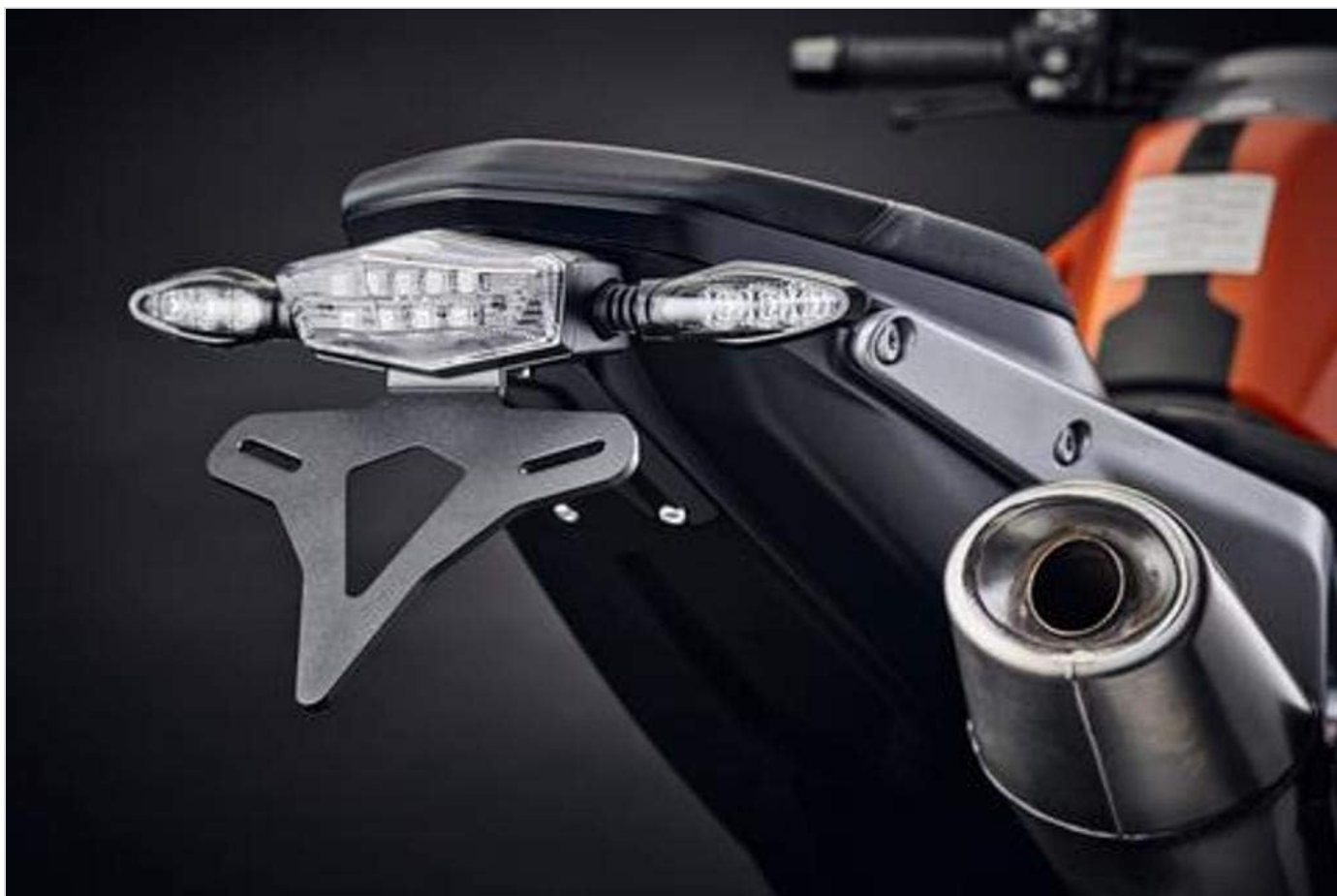
Figure 3: Side view of the tail tidy installed on a KTM Duke, highlighting the integration with the motorcycle's lines.
