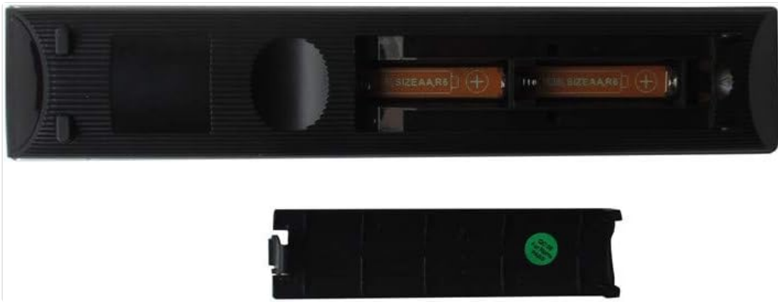
Image: Back of the remote control with the battery compartment open, revealing the slots for two AAA batteries.
