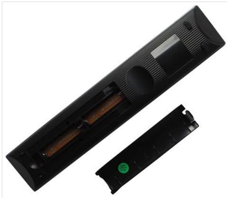
Image: Rear view of the remote control with the battery cover removed, illustrating the correct placement of AAA batteries.
