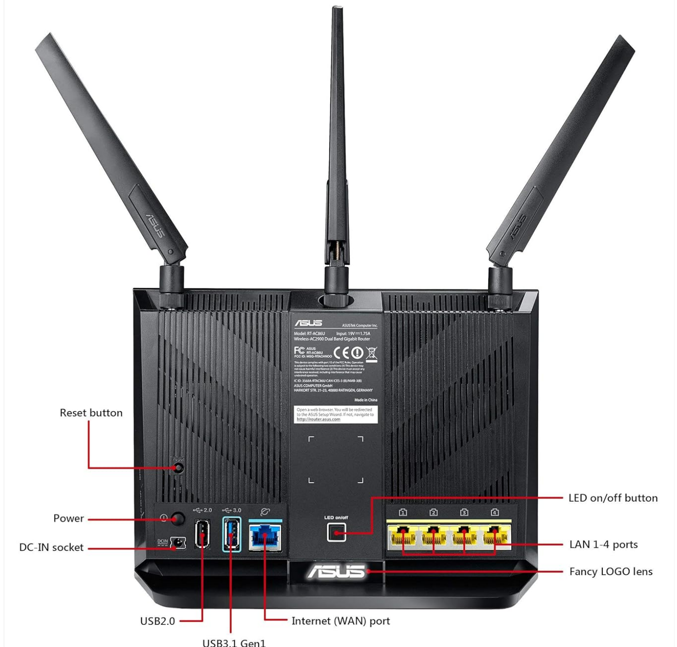
Image: Rear view of the ASUS RT-AC86U router. Labels indicate the Reset button, Power button, DC-IN socket, USB2.0 port, USB3.1 Gen1 port, Internet (WAN) port, LAN 1-4 ports, LED on/off button, and Fancy LOGO lens.
