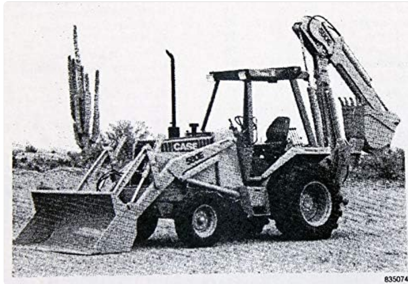
Figure 2.1: A typical Case 580 series Tractor Loader Backhoe. Always ensure the machine is in good working order before operation.
