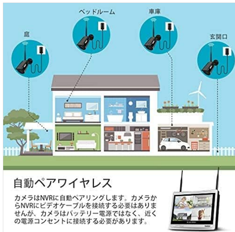
Image 3.4: Automatic wireless pairing and power connection for cameras.
