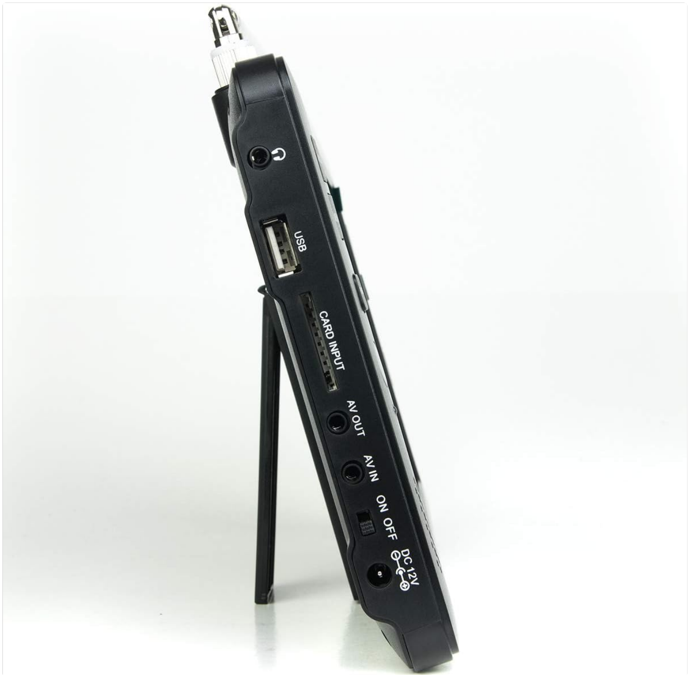
Figure 3.2: Side view of the Tyler TTV704-9 Portable TV with input/output ports.
