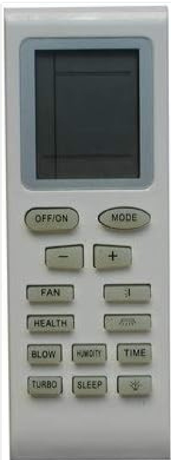
Figure 1: Front View of the Remote Control. This image displays the front of the remote control, showing the LCD screen at the top and an array of buttons including OFF/ON, MODE, temperature adjustments (+/-), FAN, HEALTH, BLOW, HUMIDITY, TIME, TURBO, and SLEEP.
