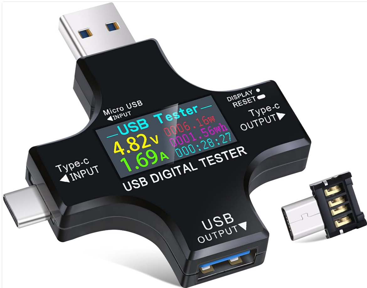
Image 2.1: Front view of the Eversame USB Tester displaying measurement data.
