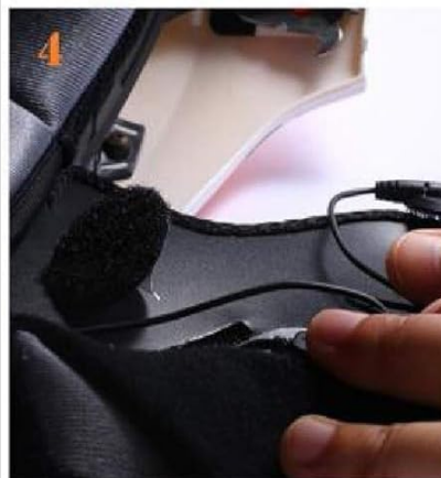
4 Remove lining, 3M glue fixed microphone or earphone
