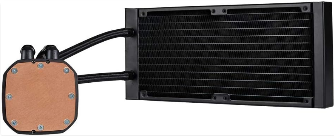
Image: The copper cold plate of the H100i RGB PLATINUM with pre-applied thermal compound.
