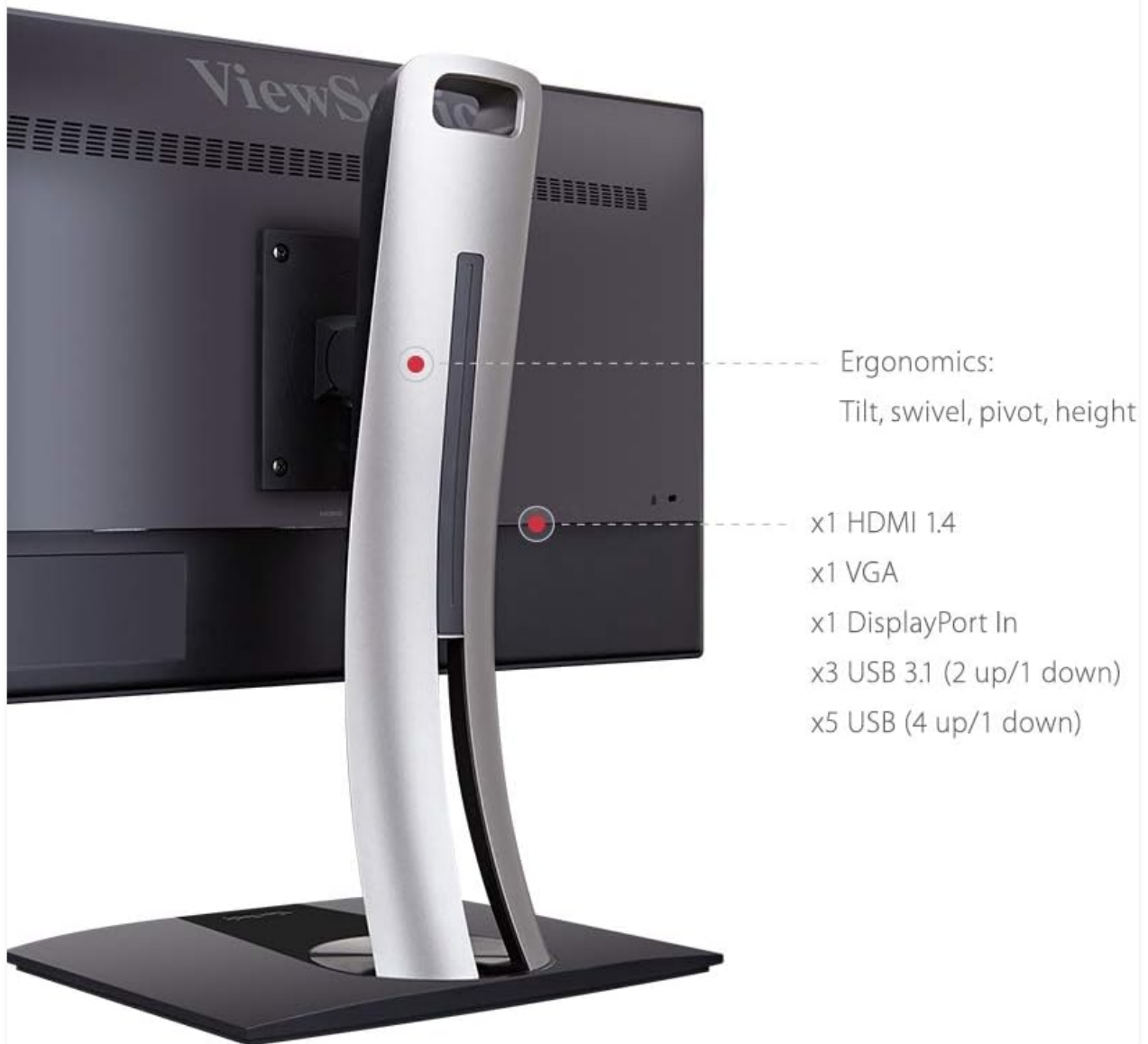
Image: Rear view of the ViewSonic VP2458 monitor, highlighting its ergonomic adjustments (tilt, swivel, pivot, height) and various connectivity ports including HDMI 1.4, VGA, DisplayPort In, and multiple USB 3.1 ports.
