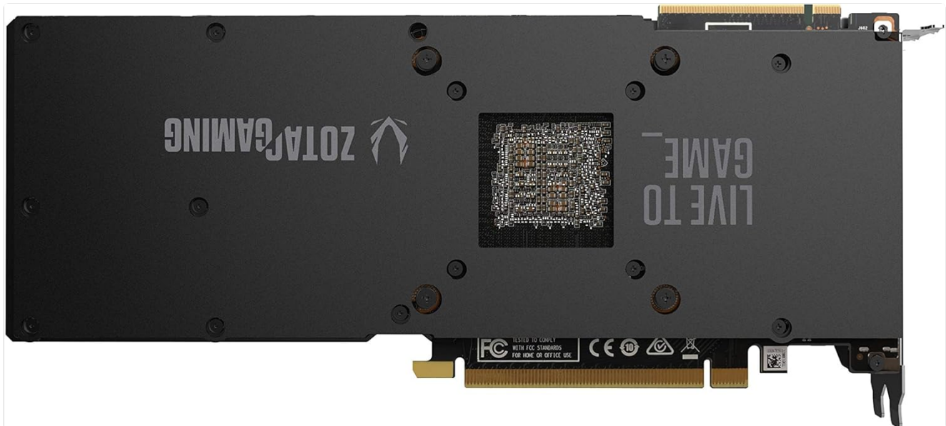
Image: Backplate view of the ZOTAC Gaming GeForce RTX 2080 Ti Blower graphics card, featuring a metal backplate for structural rigidity and heat dissipation.
