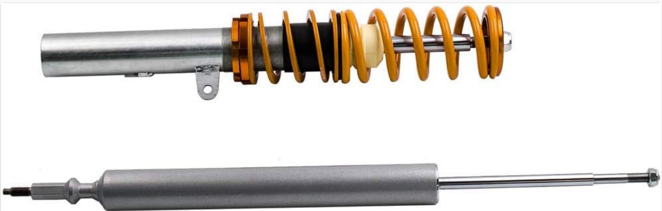
Image: An assembled front coilover unit and a separate rear shock absorber, illustrating the components before installation.
