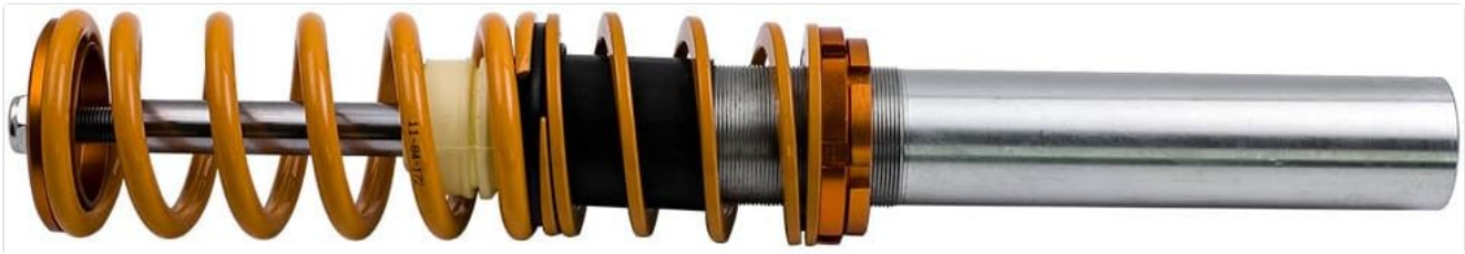
Image: A close-up view of the coilover's threaded body, spring perch, and locking collars, which are used for height adjustment.
