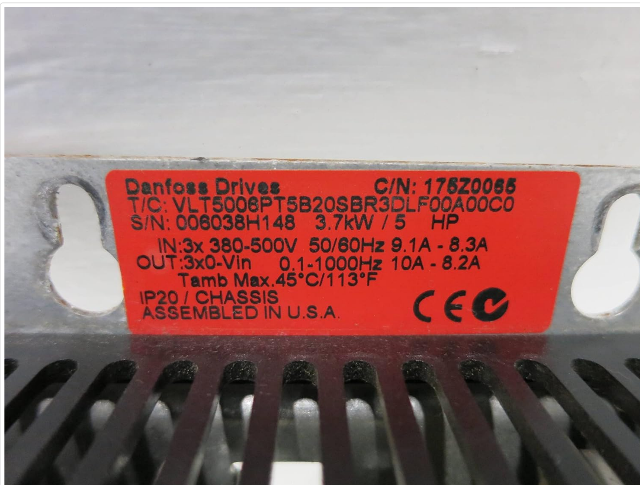
Figure 7.1: Product label for the Danfoss VLT5000 drive. This label provides critical information including the model number (VLT5006PT5B20SBR3DLF00A00C0), serial number, power ratings (3.7kW / 5HP), input/output voltage and current specifications, maximum ambient temperature (45°C/113°F), and IP20/CHASSIS enclosure rating.
