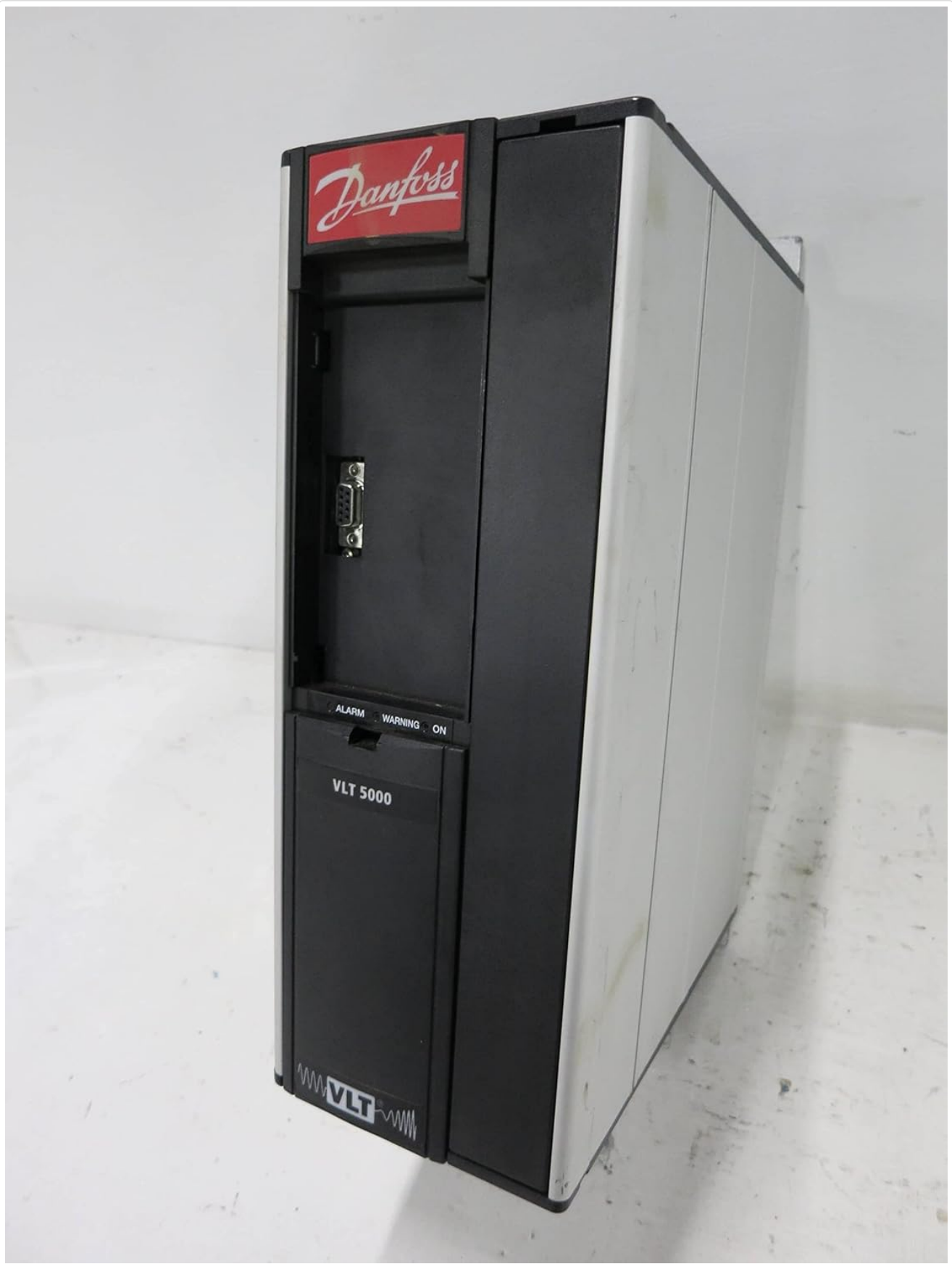
Figure 3.1: Front view of the Danfoss VLT5000 Variable Speed Drive. This image shows the main housing, the Danfoss logo, the 'VLT 5000' model designation, and indicator lights for ALARM, WARNING, and ON status.
