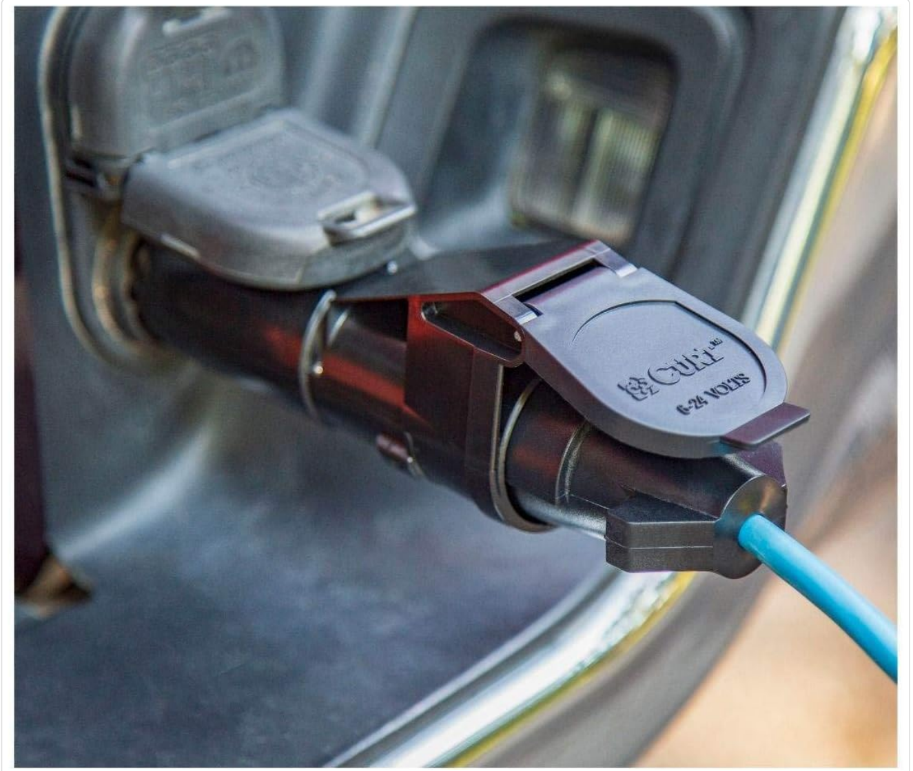
Image: The CURT Echo device securely plugged into the vehicle's 7-way trailer wiring socket, ready for use.
