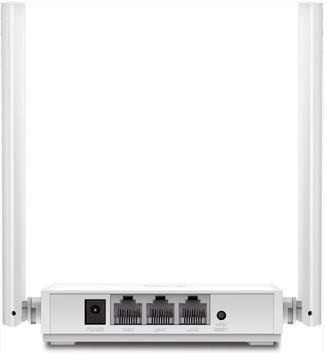
Rear view of the TL-WR820N, displaying the power input, WAN port, two LAN ports, and the WPS/Reset button.
