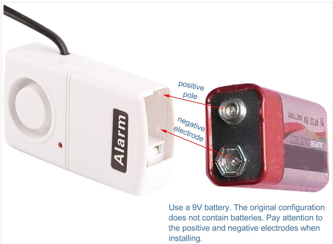
Figure 3.1: Battery Installation
