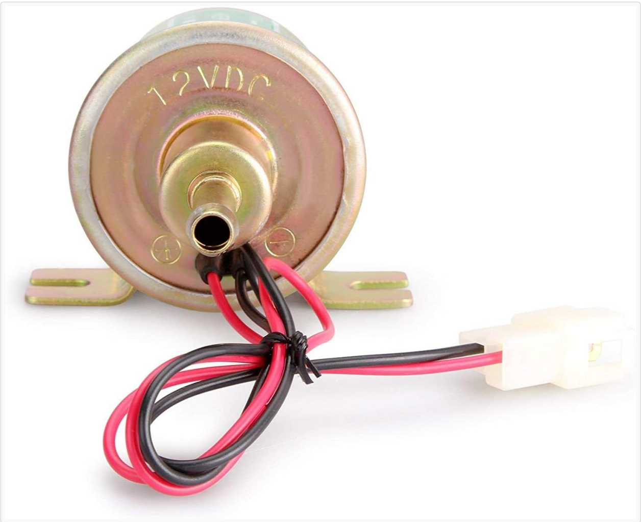
Figure 3: Rear view of the fuel pump showing the 12VDC marking and the red and black electrical wires with their connector. The red wire connects to positive, and the black wire to negative.
