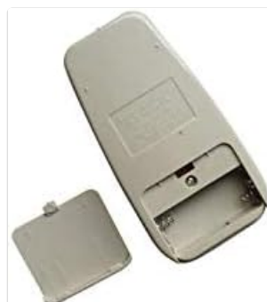
Figure 1: Back of the remote control with the battery cover removed, illustrating the battery compartment for AAA batteries.
