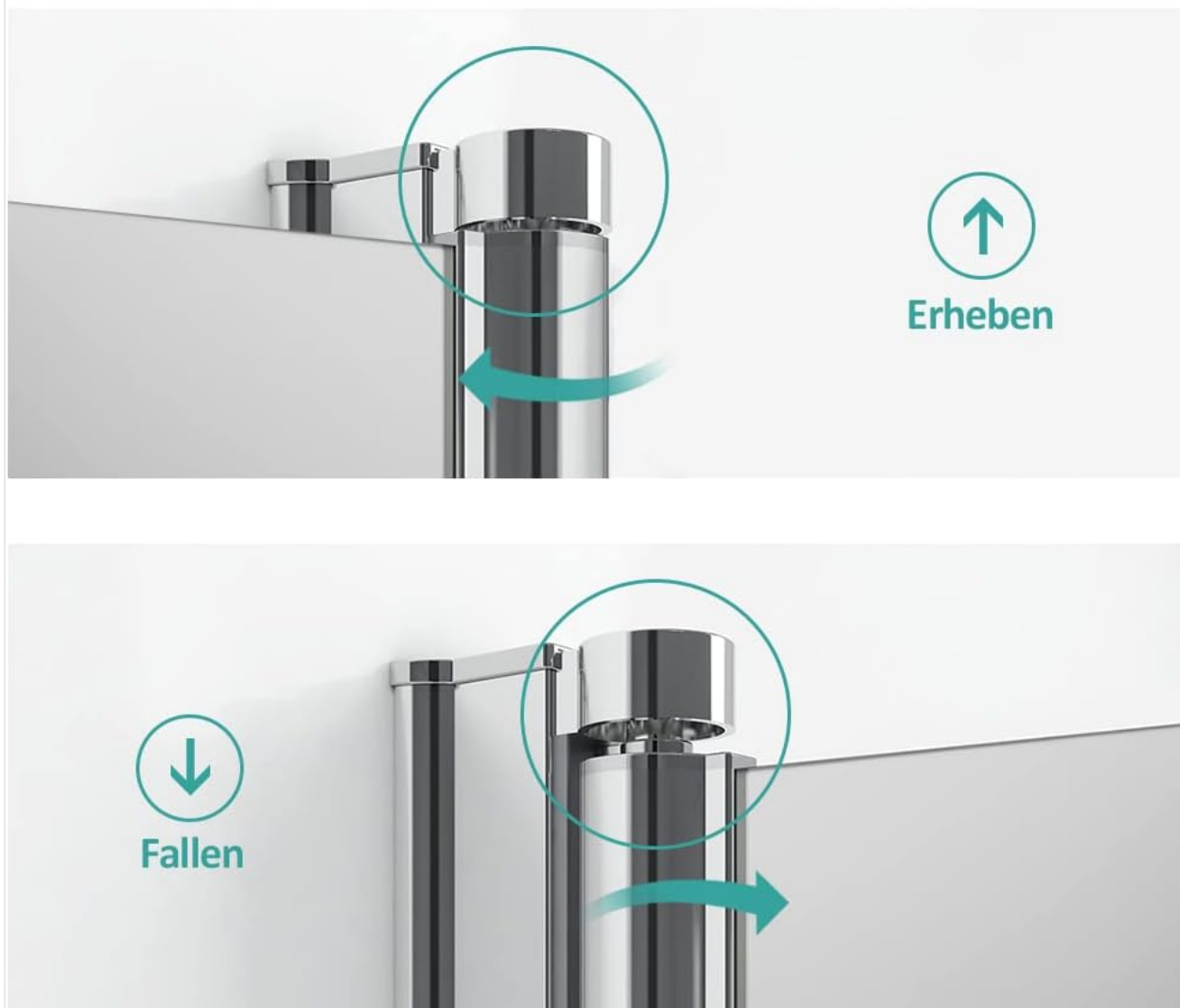
Figure 5: The 4mm lift and lower mechanism reduces noise and protects the seal from wear.
