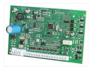
Image: The green circuit board of the DSC PC1404 control panel, showing various electronic components and terminal blocks.
