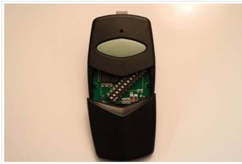
Image: The remote with its cover open, revealing the 12 dip switches and battery compartment.
