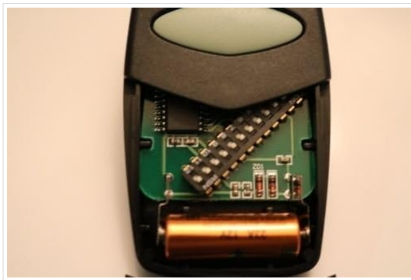
Image: A detailed view of the remote's interior, highlighting the 12 dip switches and the A23 battery.
