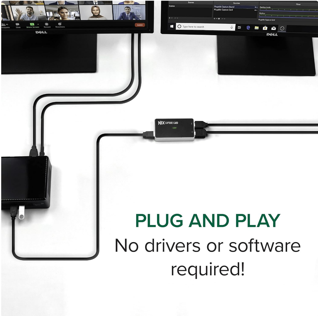
Image: The Plugable NIX Capture Card connected to a laptop via USB and an external monitor via HDMI pass-through, illustrating a typical setup.
