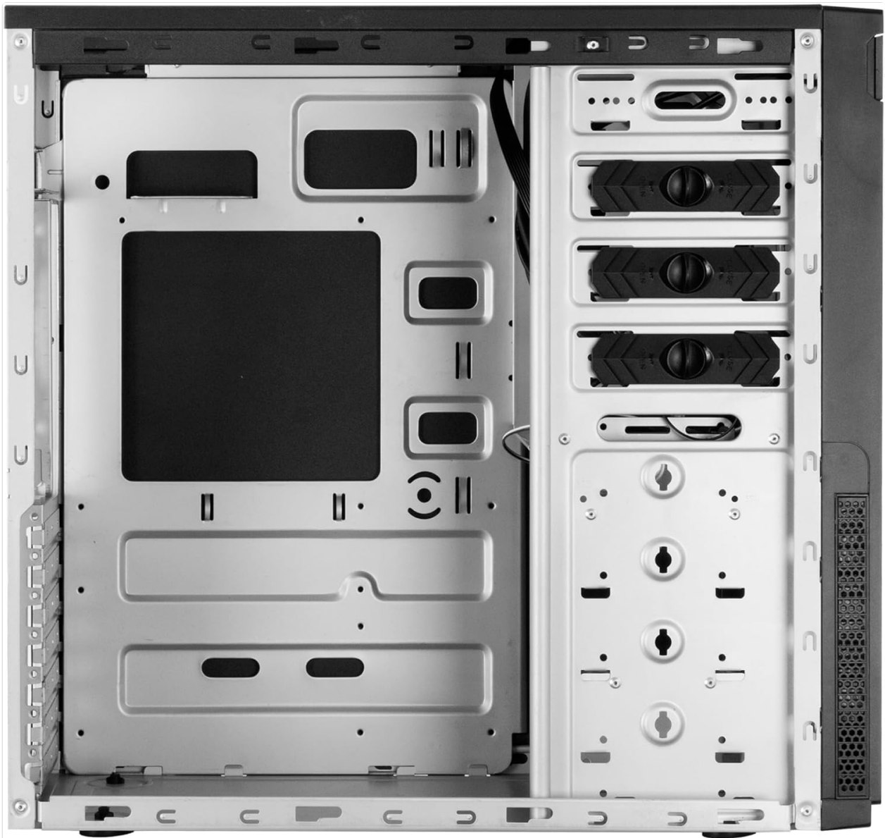
Figure 3: Internal view of the Chieftec HC-10B-OP Computer Case, showing the motherboard mounting area and drive bays. This image highlights the layout for component installation.
