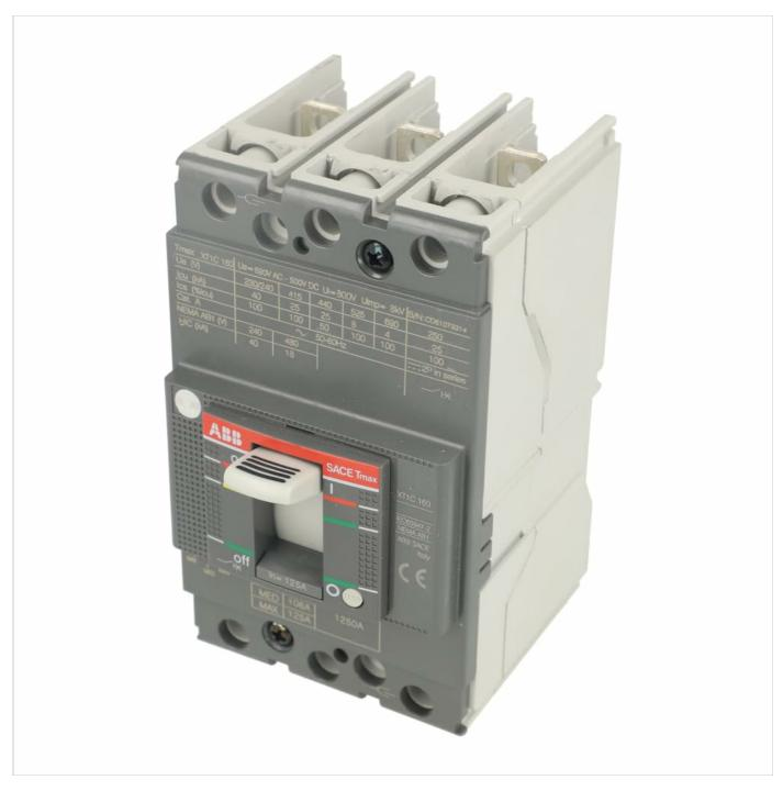
This image shows the ABB TMAX XT1C 160 circuit breaker. Key features visible include the ABB logo, the SACE Tmax branding, the 'off' position indicator, and the current rating adjustment dials (MED 106A, MAX 125A). The top section displays technical specifications such as rated operational voltage (Ue), rated ultimate short-circuit breaking capacity (Icu), and rated impulse withstand voltage (Uimp). The breaker is a 3-pole design with front terminals.
