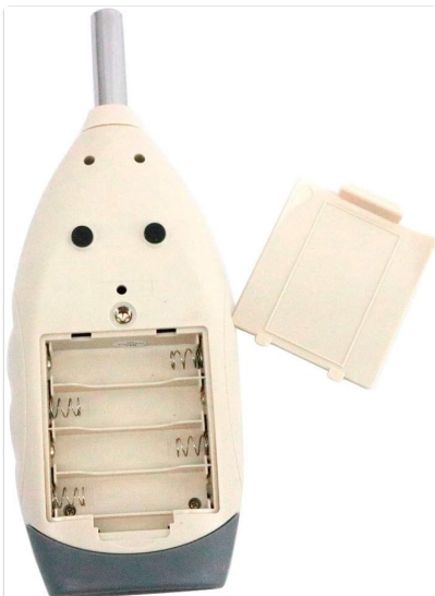
Figure 3.4: AR844 Sound Level Meter with the battery compartment open. This image illustrates the four AAA battery slots inside the compartment.
