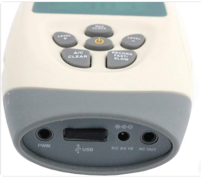
Figure 3.5: Bottom ports of the AR844 Sound Level Meter. This detailed view shows the PWM output, USB port for PC connection, DC 6V power input, and AC output ports.
