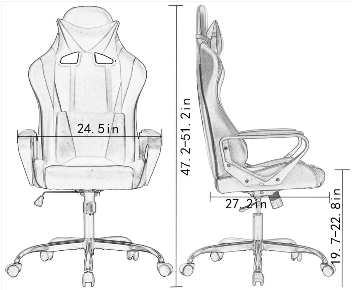
Figure 1: Chair dimensions and structural overview. This diagram illustrates the overall size and key components for assembly reference.
