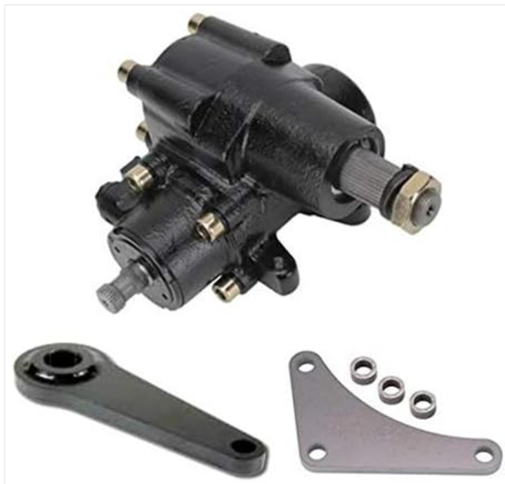
Figure 1.1: The Vega Power Cross Steering Gear Box Combo, including the gear box, pitman arm, and mounting bracket.
