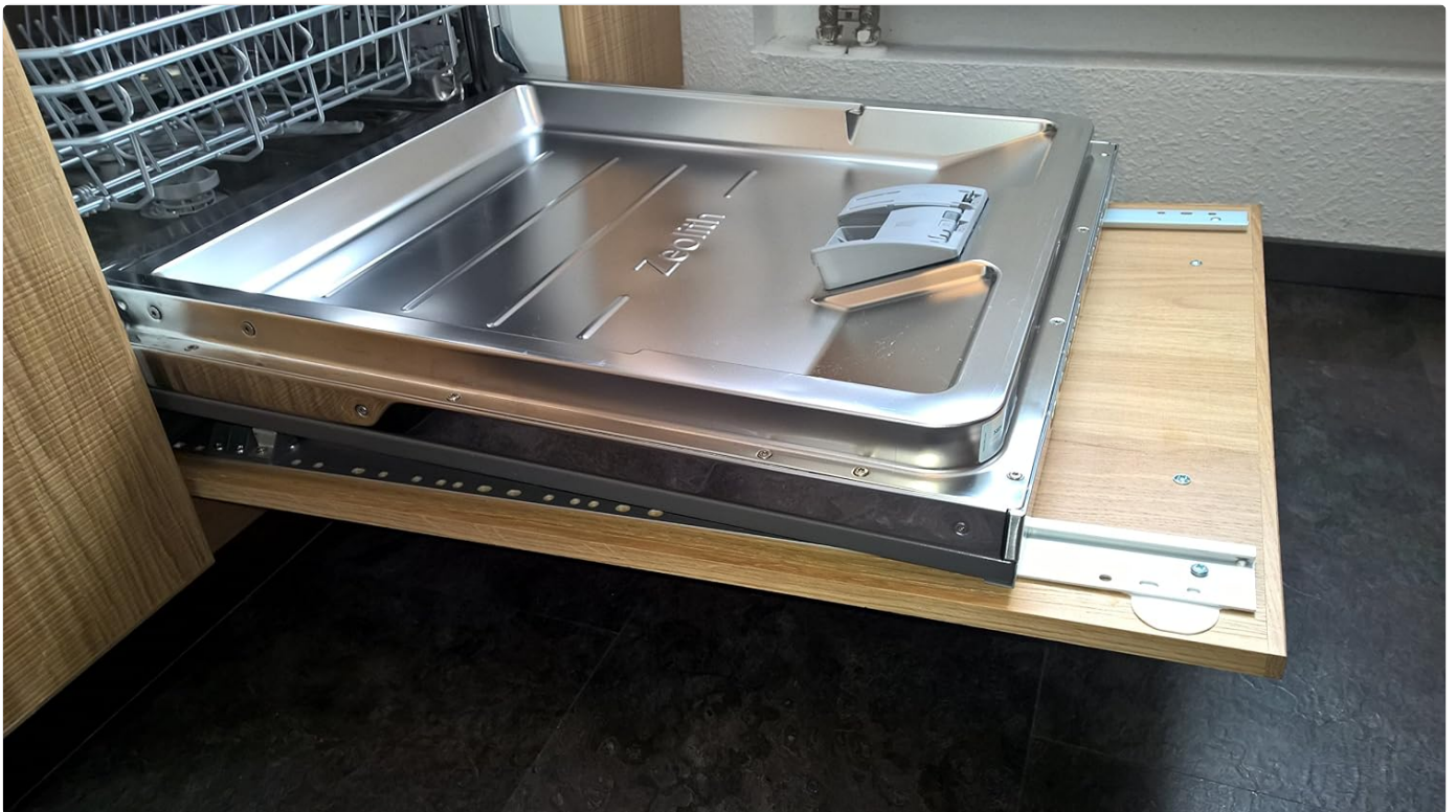
Figure 4.2: A detailed view of the sliding hinge mechanism, showing how the dishwasher's lower tray and door interact with the sliding rail as the appliance is opened.
