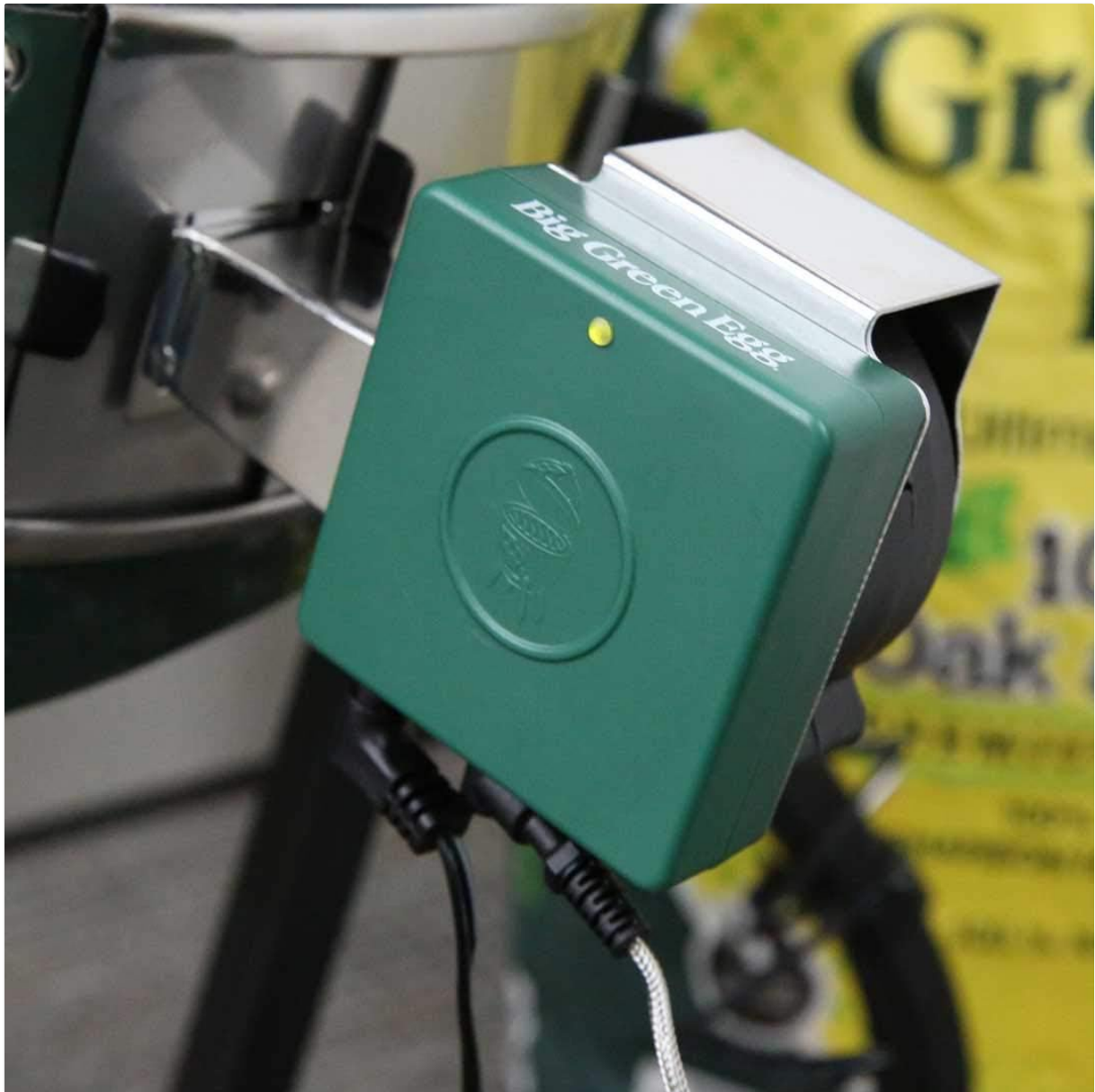
Image: The Egg Genius unit securely mounted to the lower vent of a Big Green Egg grill, with power and probe cables connected.
