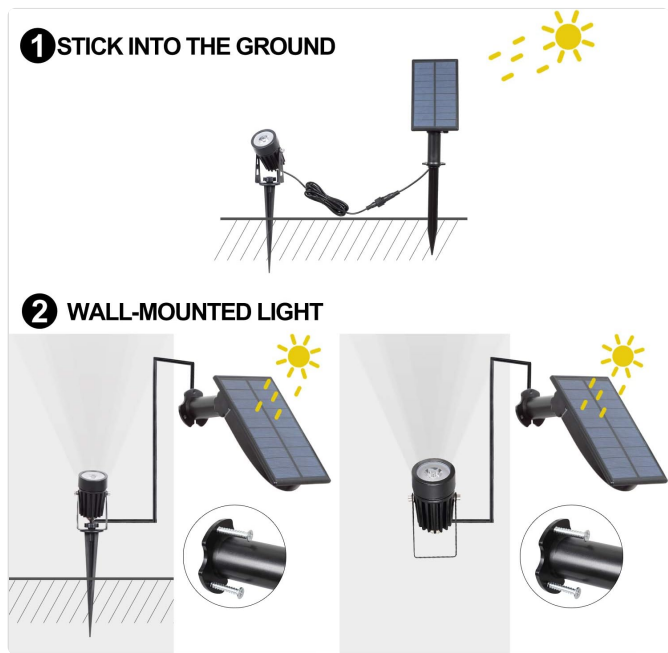
Image 4.1: Visual guide for both ground stake and wall-mounted installation methods.
