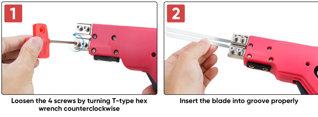
Figure 3: Loosening screws and inserting the blade.
