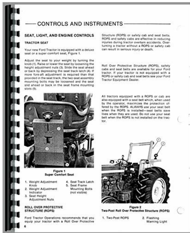
Figure 2: Illustration showing seat adjustment controls (Figure 1) and a two-post Roll Over Protective Structure (ROPS) (Figure 2) on a Ford tractor. Key components are numbered for identification.
